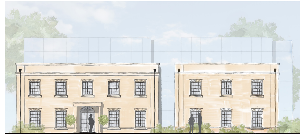
Option 2 Elevation Traditional Georgian style building with a modern twist - mirror glazed material on top floor to soften roof level.
